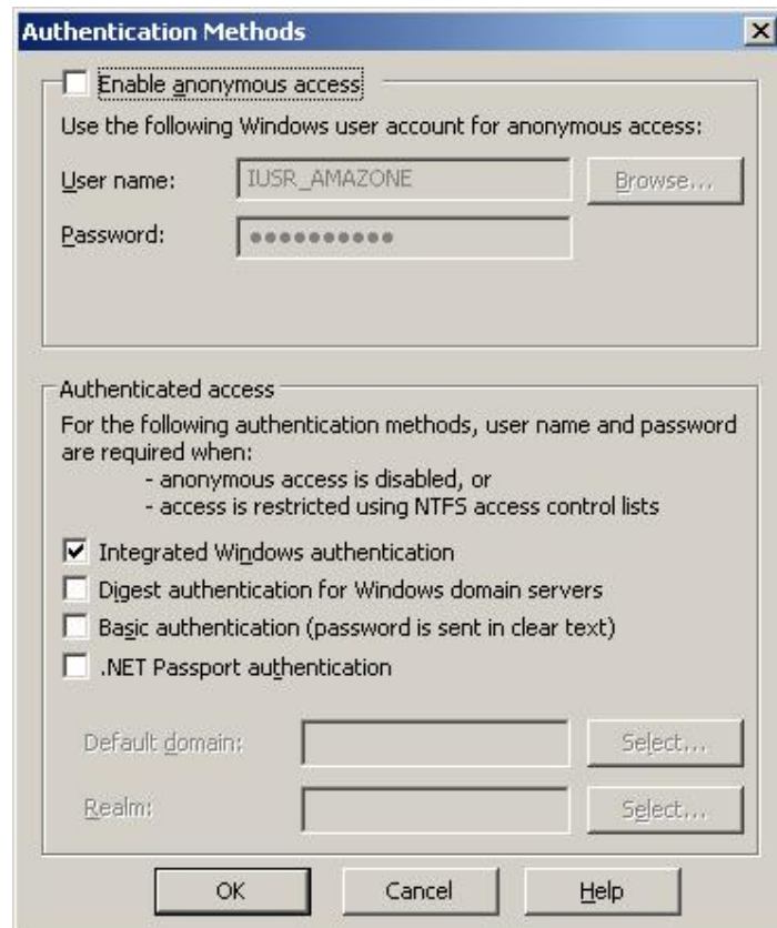
Figure 13: Specify the Authentication method: Disable anonymous access and enable integrated Windows authentication.
